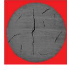
4 rating - FAIL More than eight internal cracks, or one or more cracks longer than 80% of the cross section.
