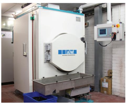
Yet another enhancement of our facilities has been seen with the addition of a new state-of-the-art machine to undertake cryogenic cleaning and de-flashing.
