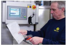
run fully customised multiple programmes linked to our own management systems. The operator simply has to scan the docket accompanying each batch of components and the unit automatically selects the appropriate programme for the part, thereby ensuring quality control and traceability are maintained throughout the process.
