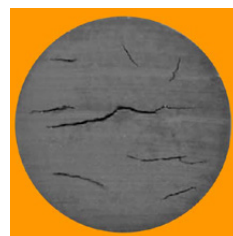
3 rating - PASS Less than nine internal cracks, of which a maximum of two cracks can have a length between 50% and 80% of the cross section.
